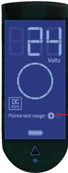
Example of 24 V DC detection, display is BLUE because < 50 V.
