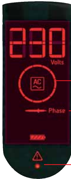
Example of detecting 230 V AC, displayed in RED .
