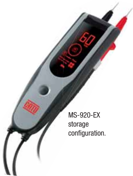
Example of detecting 230 V AC, displayed in RED .
